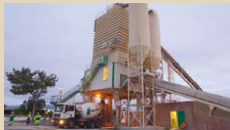
Production of self-compacting Ductal® in a ready-mix plant and application on site
